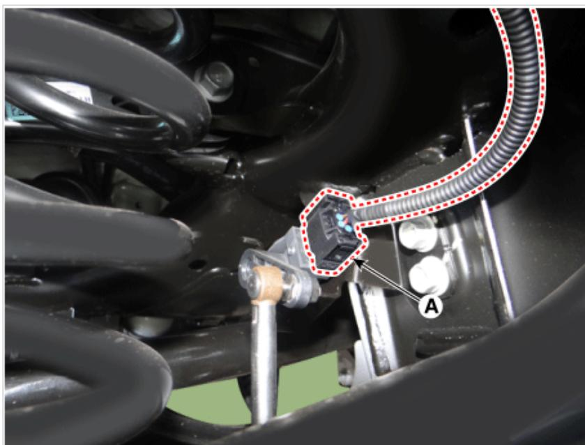
3. Remove the headlamp leveling unit mounting link (A).
