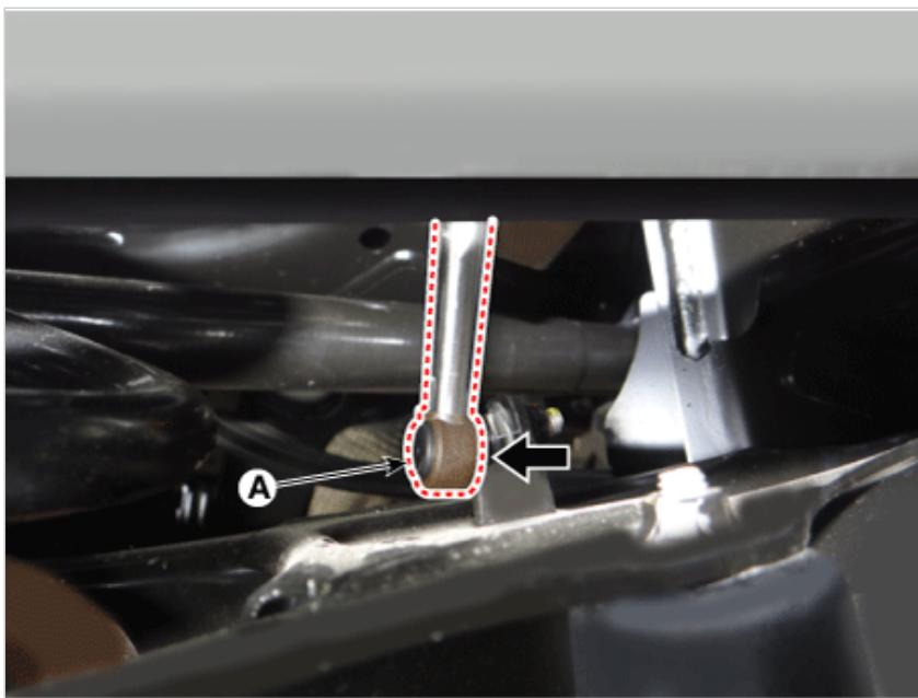
4. Remove the headlamp leveling unit (A) after loosening the mounting bolts.
